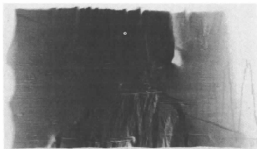
Fig. 6. A transmission topograph of a MBANP crystal showing near-perfect lateral sectors and upper and lower sectors with a high number of defects.
